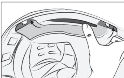
Finally, insert the plastic clips into the designated spaces.
