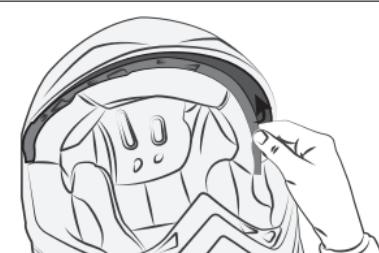
Insert the plastic part into the designated slots along the plastic frame.
