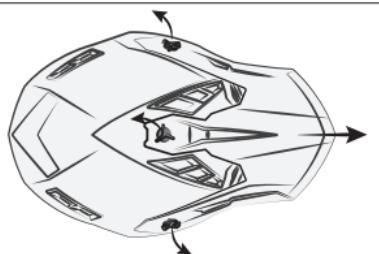
Remove the three screws and washers on the face shield.
