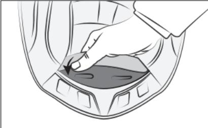
on the back of the helmet fasten the two plastic buttons.
