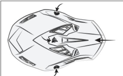
Place the face shield and secure it using the screws and washers.
