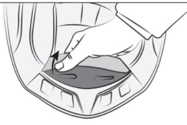
Remove the back lining by pulling the rear section to release the plastic buttons.
