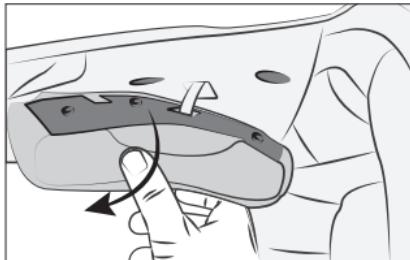
Pull by unfastening the buttons securing the cheek pad and remove it.
