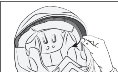
Remove the front by gently releasing the inside along the frame. To facilitate the operation, start from the side of the frame.
